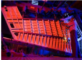
Assembly of Vertical Fin for the Sukhoi-30 FKG Fighter Bomber
